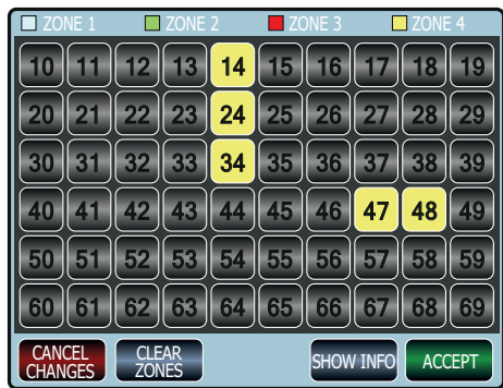
Fig. 13 – Zones setup for four individual NAUCON-1000. Scoreboards with three sideboards and two shot clocks. Referring to the drawing, Fig. 12 on the previous page.
